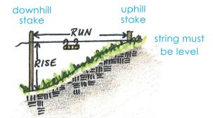
Figure 1. Determine the slope of the landscape before digging.
