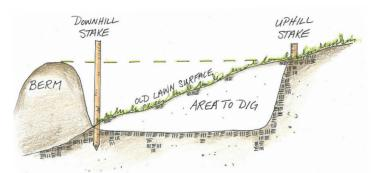
Figure 2. Where to dig and put the soil on a sloped site.
