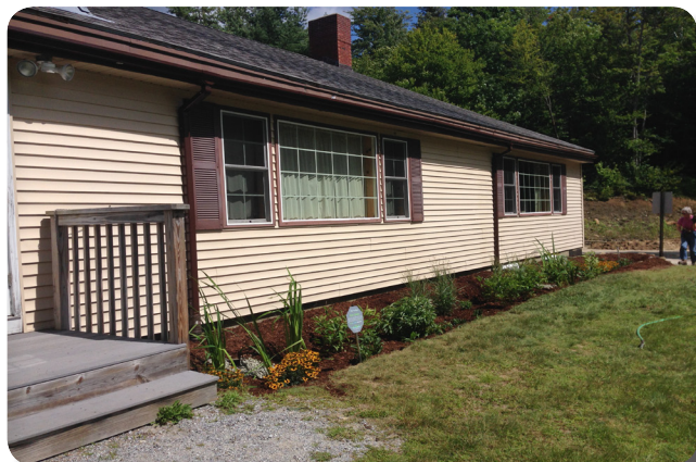
The finished rain garden receives runoff from the roof of the Camp Morgan Lodge to water the perennial plants.
