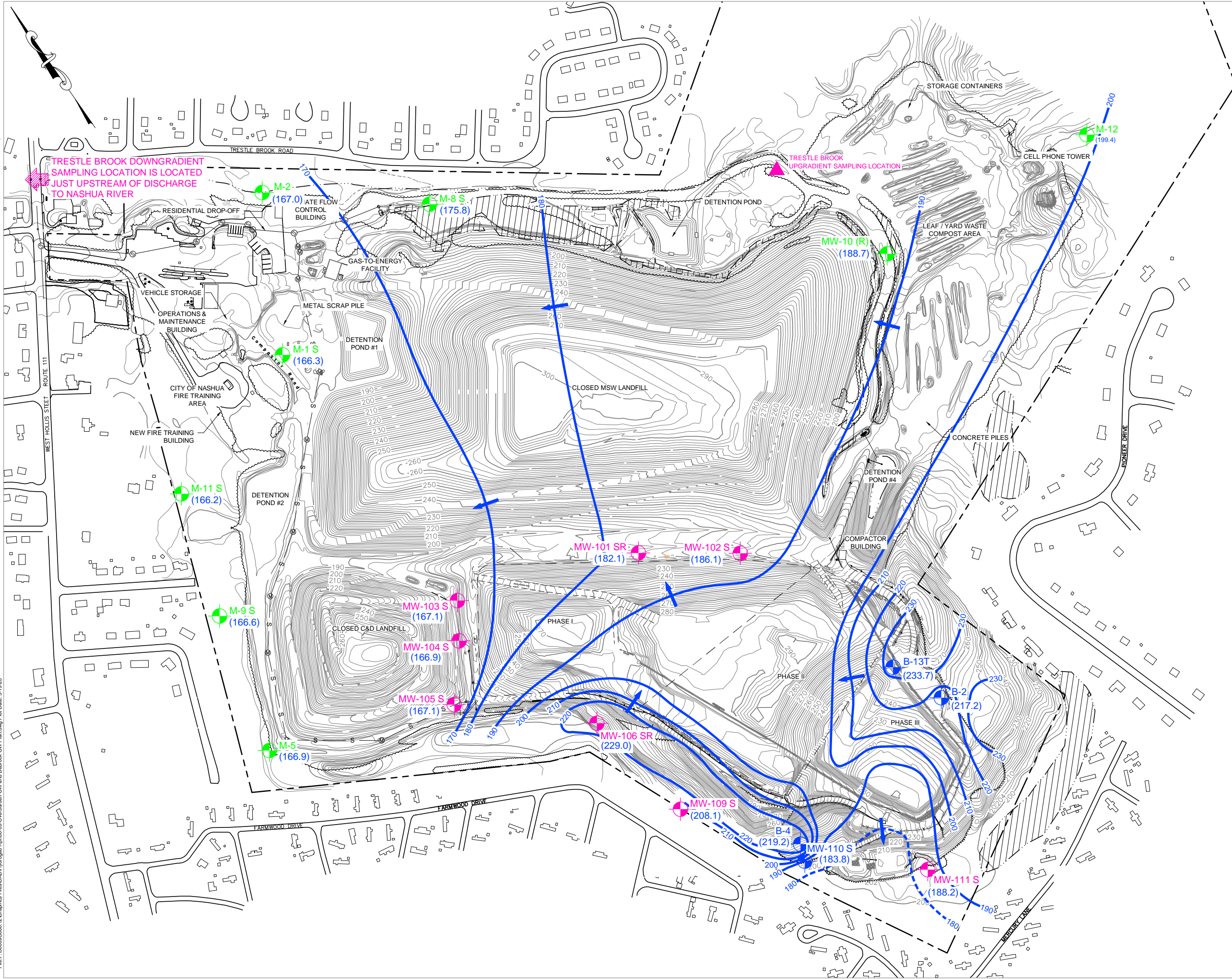
Figure 8 Four Hills Landfill Overburden Groundwater Elevation Contour Plan Hydrogeologic Report Phase IV Secure Landfill Expansion Four Hills Landfill City of Nashua, New Hampshire Nashua, New Hampshire
