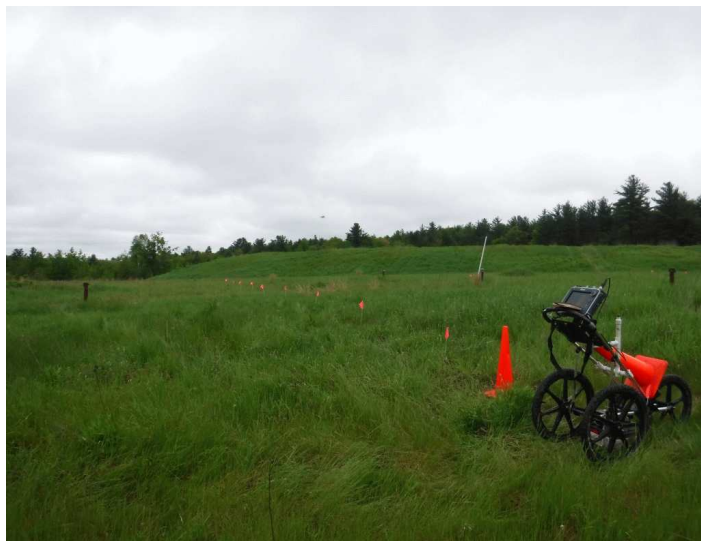
Photo 1. Typical site conditions in the geophysical survey area. GPR system at right.
