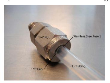
5. For the other end of the FEP, slide on another ½" SwageLok nut and ½" nylon ferrule. Insert the end of the FEP into a ¼ "to ½" SwageLok® reducer. Using a ½" and ½" wrench, tighten the nut as before. Be careful to keep the FEP seated tightly into the fitting while tightening.
