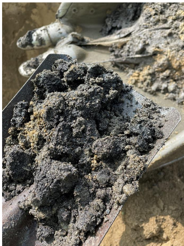
Photos 2 & 3: Gray, black stained soil with oil sheen and odor.
