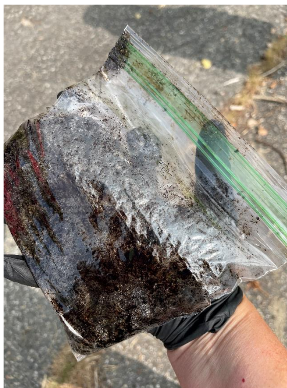
Photo 4: Discrete sample of stained soil sample collected for field screening, oil as free product observed in plastic bag.
