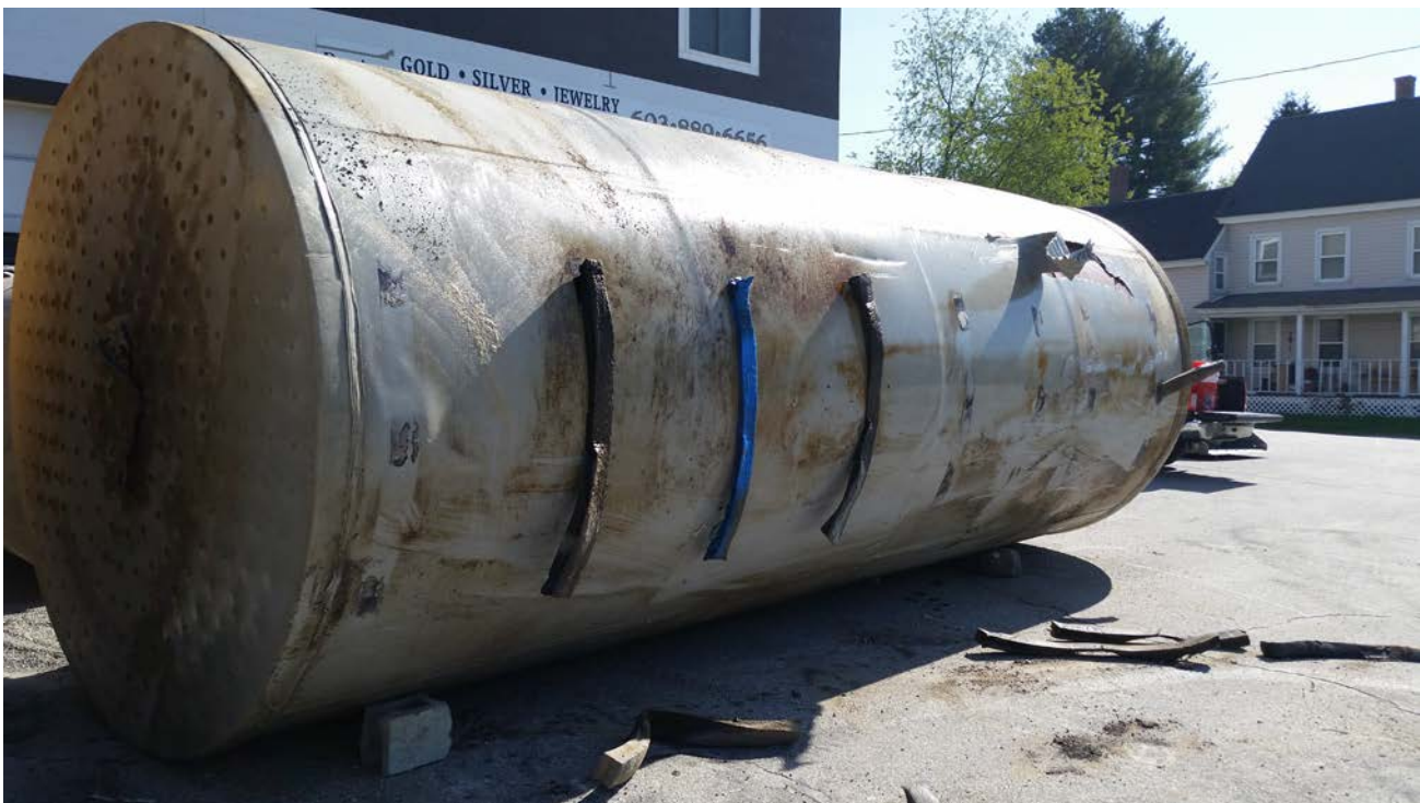
5. 8000-gallon Gasoline UST following removal; no rips, holes or tears were noted (note plastic welded containment around tank).
